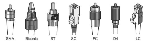
Figure 3-21 Common Fiber-Optic Connector Types
