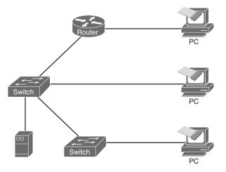
Figure 3-2 Typical Components of a LAN
