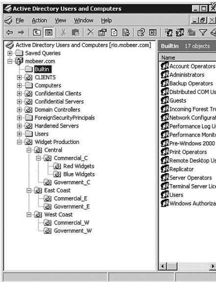
**FIGURE 3.1** The hierarchical structure of OUs in an Active Directory domain.
