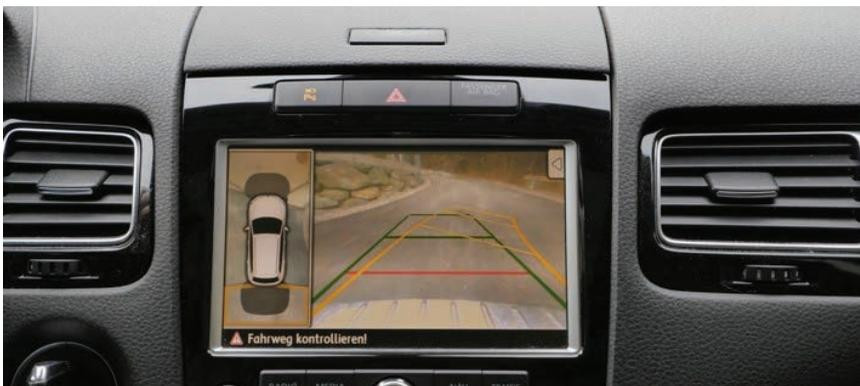
**Figure 1.23** The parking assistant is a commercially available AR feature in many contemporary cars. Courtesy of Brigitte Ludwig.
