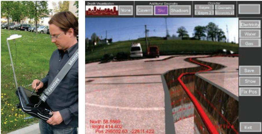
**Figure 1.14** Tablet computer with differential GPS system for outdoor AR (left). Geo-registered view of a virtual excavation revealing a gas pipe (right). Courtesy of Gerhard Schall.
