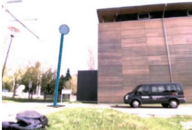
**Figure 1.15** While the drone has flown far away and is barely visible, its position can be visualized using a spherical AR overlay. Courtesy of Stefanie Zollmann.
