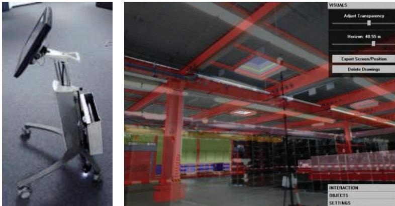
**Figure 1.13** The Planar is a touchscreen display on wheels (left), which can be used for discrepancy analysis directly on the factory floor (right). Courtesy of Ralph Schönfelder.
