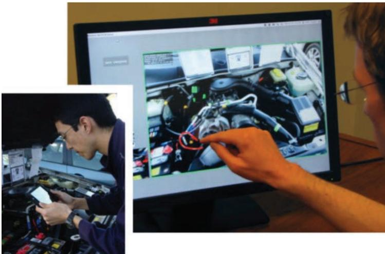
**Figure 1.18** A car repair scenario assisted by a remote expert via AR telepresence on a tablet computer (top). The remote expert can draw hints directly on the 3D model of the car that is incrementally transmitted from the repair site (bottom). Courtesy of Steffen Gauglitz.
