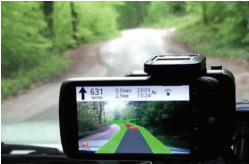
**Figure 1.22** Wikitude Drive superimposes a perspective view of the road ahead. Courtesy of Wikitude GmbH.
