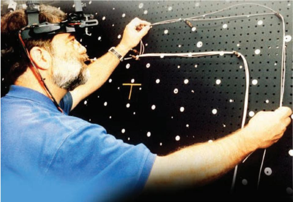
**Figure 1.3** Researchers at Boeing used a see-through HMD to guide the assembly of wire bundles for aircraft. Courtesy of David Mizell.
