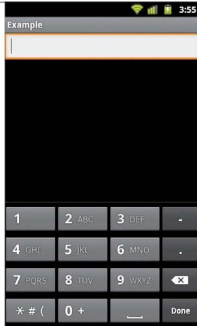
FIGURE 4.3 The keyboard displayed when the inputType of an EditText is set to phone
