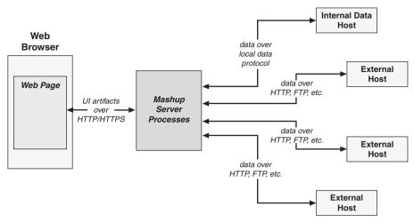
Figure 1.4 Flow of data in an out-of-process mashup
