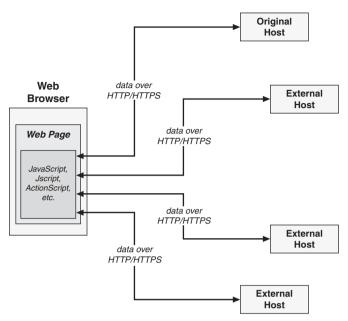
Figure 1.3 Flow of data in an in-process mashup
