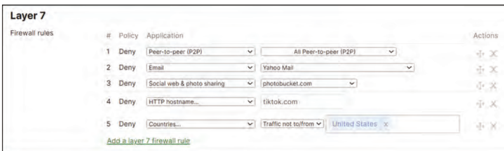
Figure 3-18 An Example Set of Layer 7 Firewall Rules Utilizing Several NBAR-Based Application Rulesets
