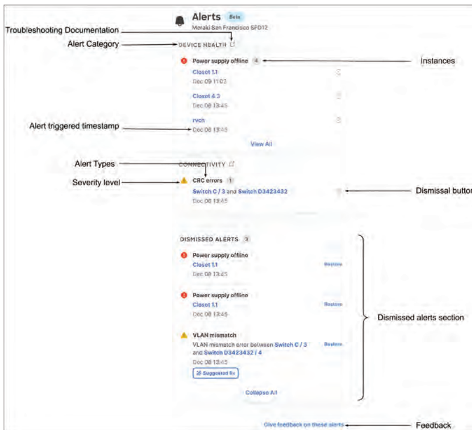
Figure 3-13 The Alert Hub Notification Panel for the Cisco Meraki San Francisco Campus Network
