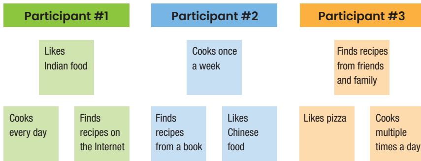
FIGURE 2.24 The first step in affinity mapping is to write down each observation for each participant and put them on a board.
