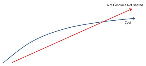
**FIGURE 3-2** As a rule, costs rise as you share fewer resources in the cloud. However, at some point, the cost begins to level out but never becomes completely flat, or diminishing.
