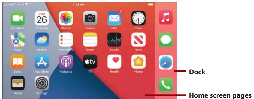
When you hold a model that supports split-screen horizontally and move to the Home screen, the Dock moves to the right side of the screen, and you see the Home screen's pages in the left part of the window. Though this looks a bit different, it works the same as when you hold an iPhone vertically.
