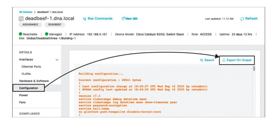
Figure 15-1 The Export CLI Output allows you to export the configuration of a device
