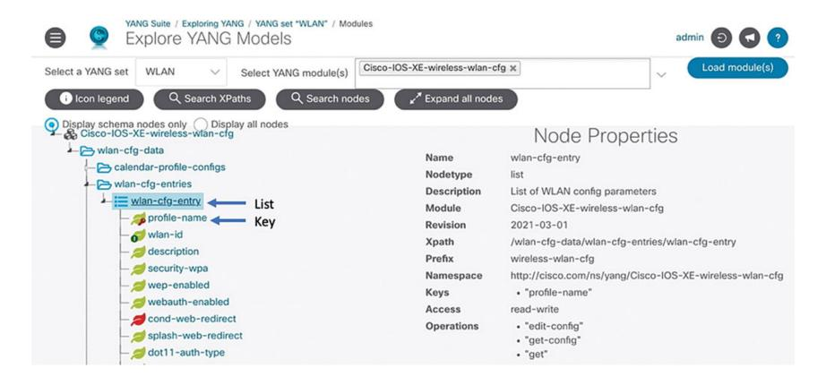
Figure 12-28 List and key in the WLAN config entry model
