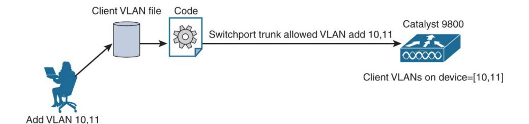
Figure 12-3 Adding client VLANs using the imperative model
