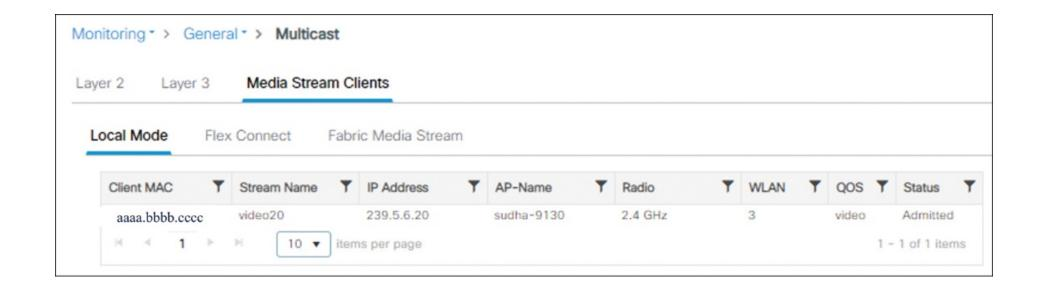
Figure 8-19 Monitoring a client admitted to the MC2UC Media Stream
