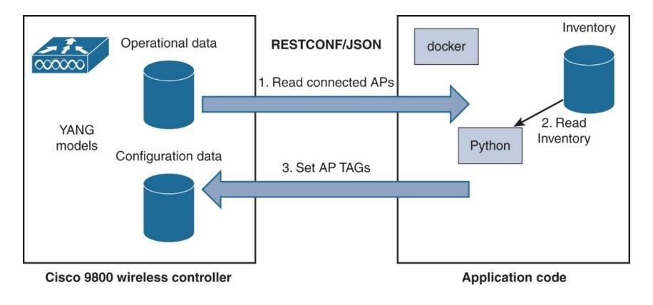
Figure 12-33 Python application to assign a tag based on the AP serial number
