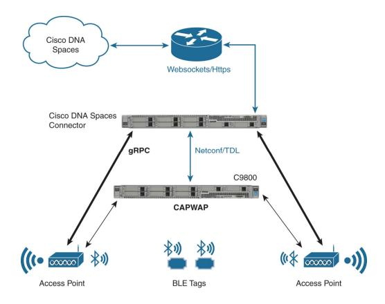
Figure 11-3 Cisco DNA Spaces Bluetooth telemetry architecture
