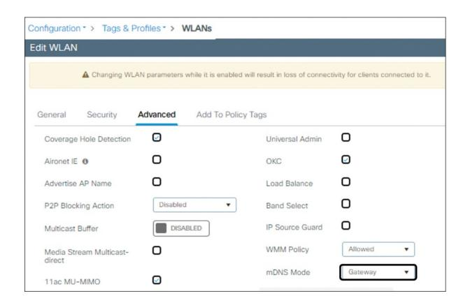
Figure 8-23 Enabling the MDNS gateway on the WLAN
