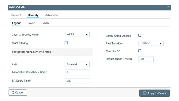
Figure 5-30 SAE WLAN example configuration
