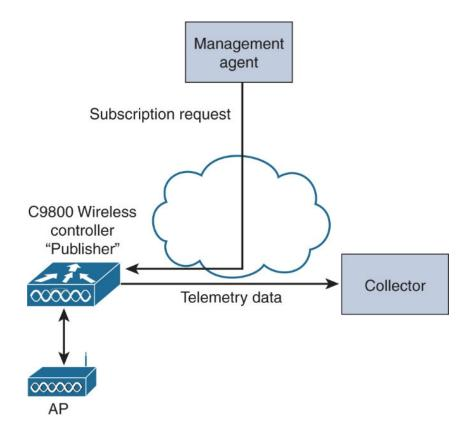
Figure 13-1 Roles in model-driven telemetry
