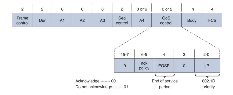
Figure 9-4 The UP (802.1D) bits in the 802.11 header
