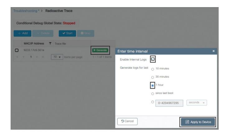
Figure 16-8 Collecting internal radioactive traces from the C9800 GUI
