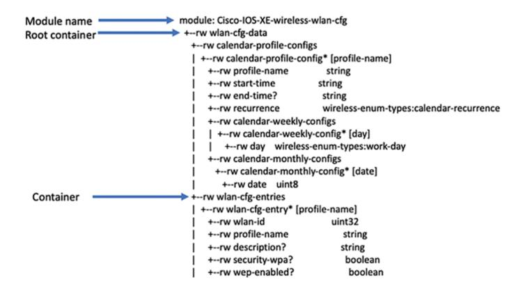
Figure 12-24 WLAN YANG Model
