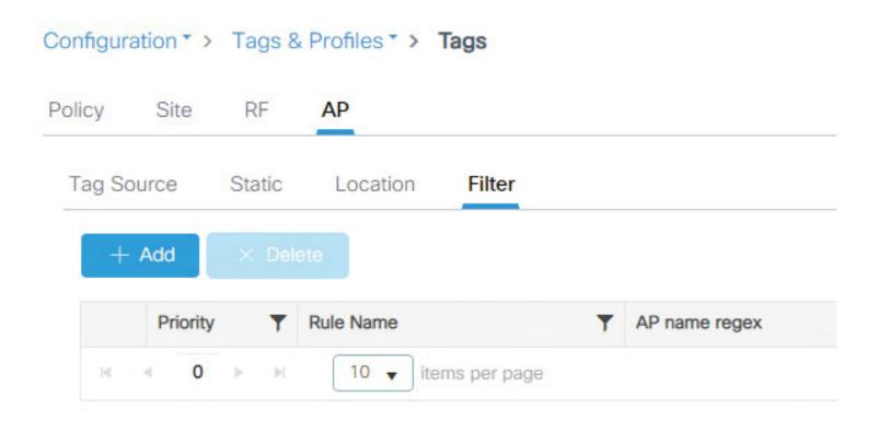
Figure 3-10 Go to the Filter tab to define the tag filter
