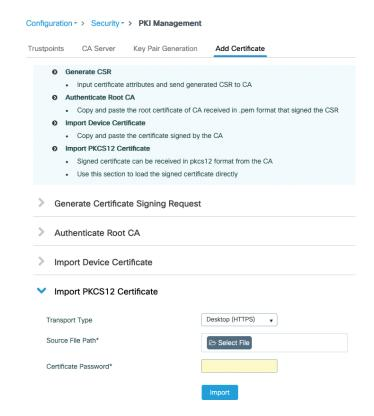
Figure 5-12 Adding a certificate chain in PKCS12 format to the WLC
