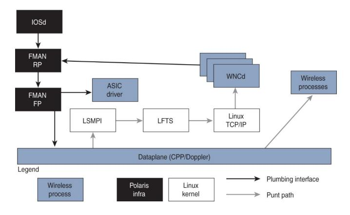
Figure 2-8 Control Plane packet processing
