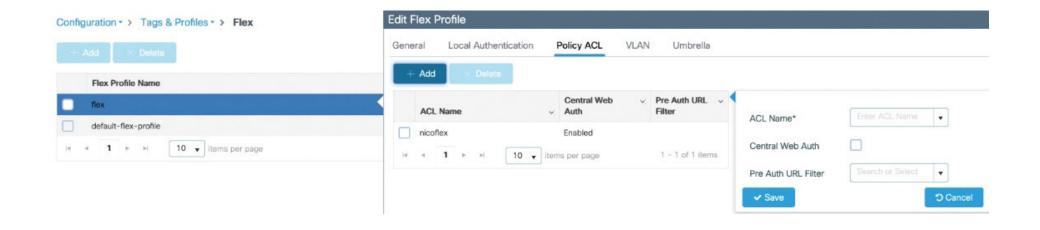
Figure 5-4 The Flex profile Policy ACL tab allows you to download ACLs to the APs
