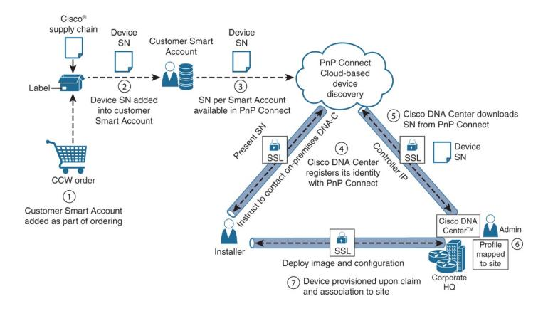
Figure 4-13 AP end-to-end onboarding process with PnP
