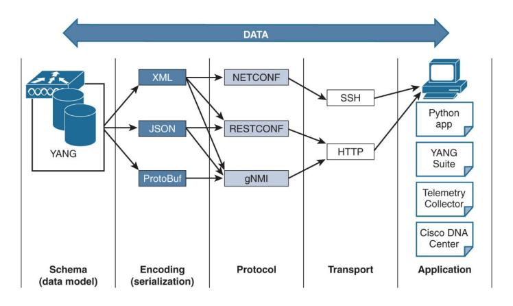
Figure 12-9 Protocols, encoding, and transport
