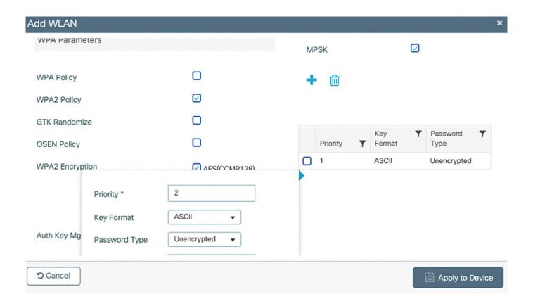
Figure 5-25 MPSK configuration in WLAN settings
