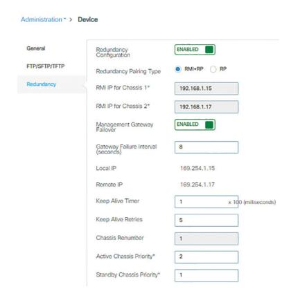
Figure 10-6 Configuring SSO redundancy on a C9800
