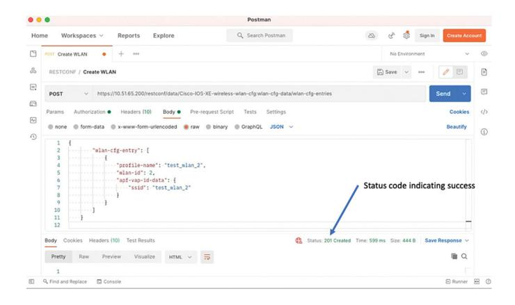
Figure 12-30 Adding a new WLAN using Postman
