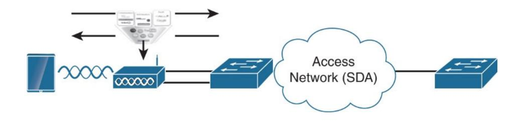
Figure 9-30 AVC in FlexConnect local switching and SDA wireless is applied at the AP
