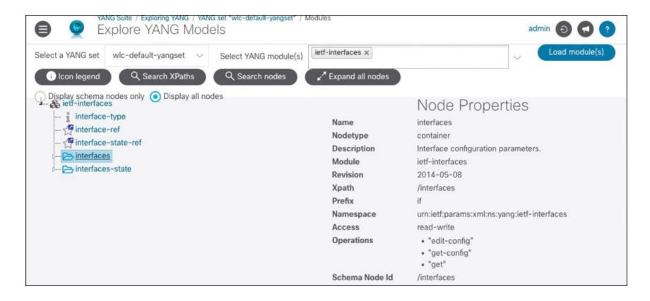
Figure 13-4 Configuration container for interfaces
