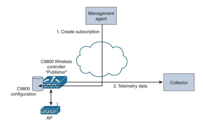
Figure 13-14 Flow for dial-out telemetry subscriptions
