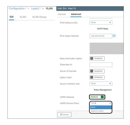
Figure 8-28 Enabling the mDNS gateway on a VLAN SVI
