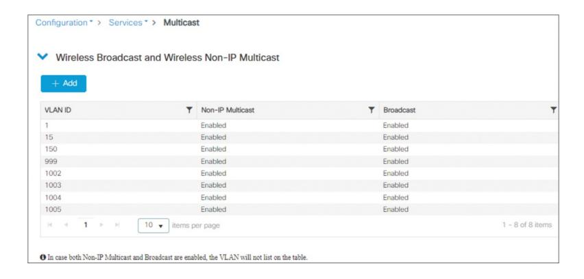
Figure 8-12 Default settings of wireless broadcast and non-IP multicast per VLAN when wireless multicast is enabled
