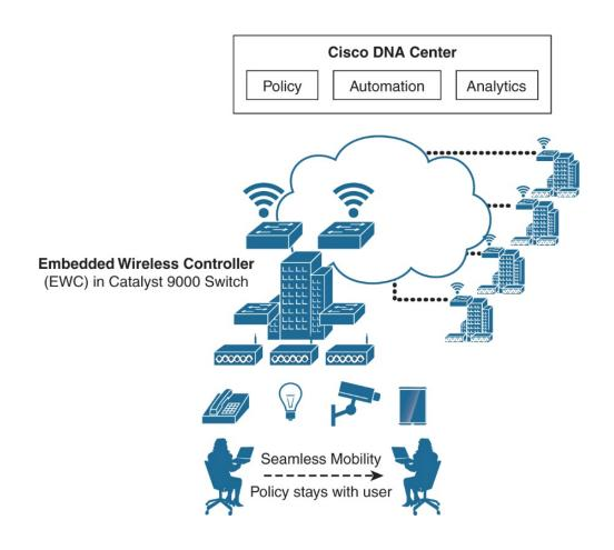
Figure 4-7 Cisco Embedded Wireless Controller (EWC) in Catalyst 9000 switches for SDA
