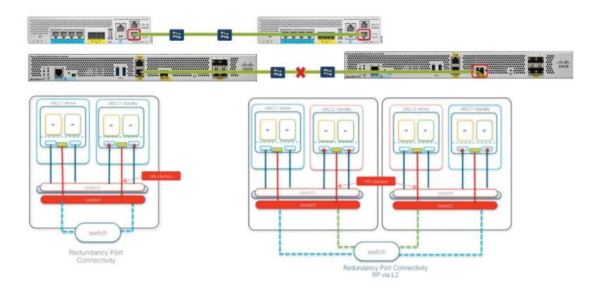
Figure 10-3 RP-to-RP connectivity between two C9800-L-Cs, two C9800-40s, and two C9800-CLs
