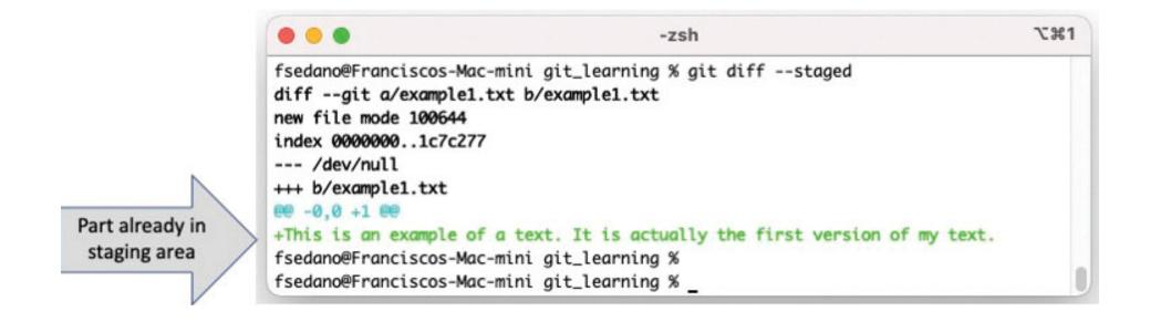
Figure A-8 Git displaying staged files
