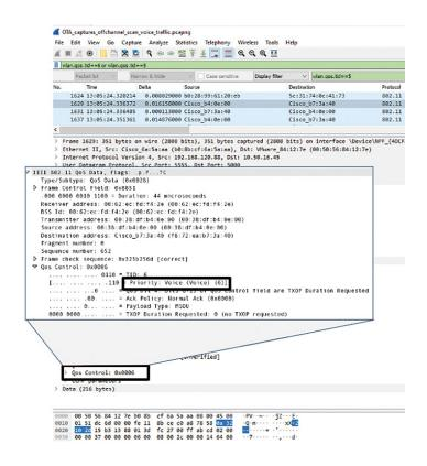
Figure 9-5 The UP value in a real over-the-air capture
