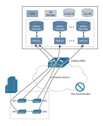
Figure 3-16 APs to WNCd distribution using the default-site-tag
