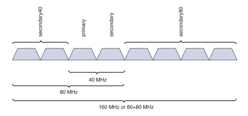
Figure 7-14 Complex primary and secondary channel plans for various channel widths
