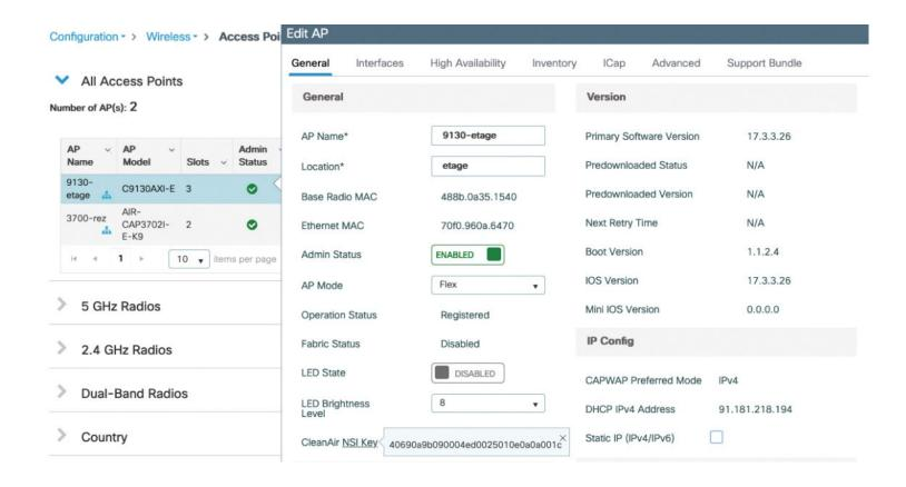
Figure 7-23 Obtaining the CleanAir key for a given AP
