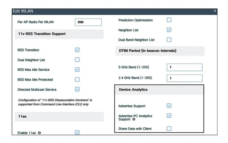
Figure 14-13 Advanced WLAN settings page, allowing you to enable Device Analytics on the C9800
