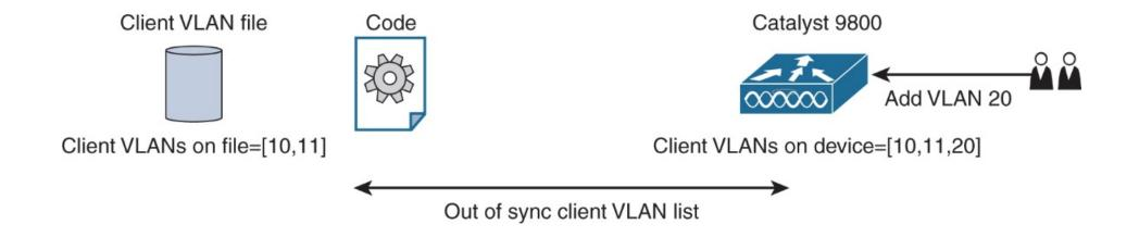
Figure 12-4 Inconsistency by using imperative models
