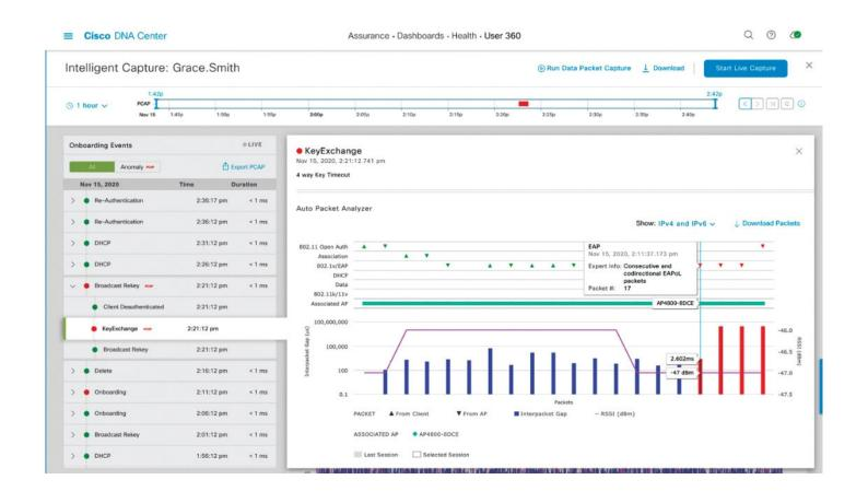
Figure 14-19 The packet analyzer from the onboarding events list
