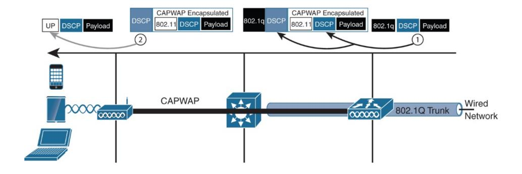
Figure 9-16 "Trust" DSCP in the downstream direction
