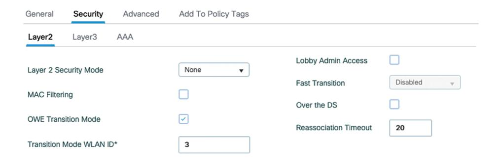
Figure 5-43 Regular open SSID linked with transition mode to an Enhanced Open SSID
