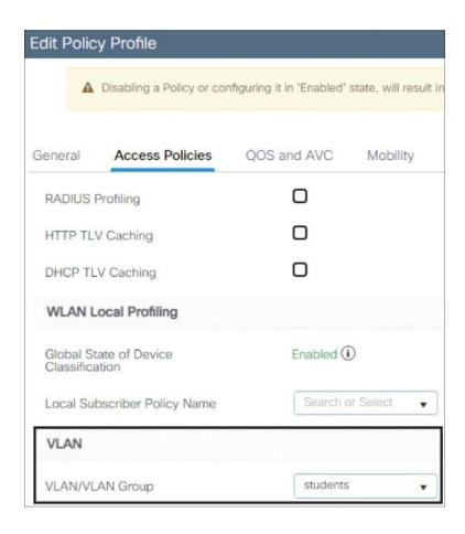
Figure 3-15 VLAN group assignment within the policy profile
