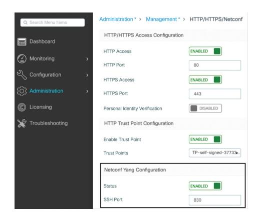
Figure 1-15 Enabling NETCONF on the Catalyst 9800 GUI
