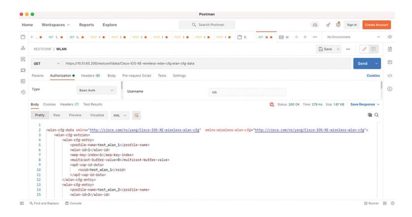
Figure 12-26 Using Postman to retrieve a list of WLANs
