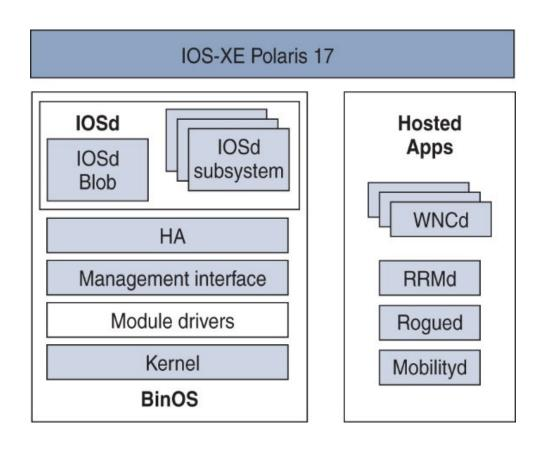
Figure 2-1 IOS-XE general software architecture
