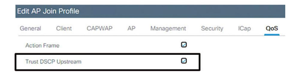
Figure 9-34 Trust DSCP settings under the AP Join Profile
