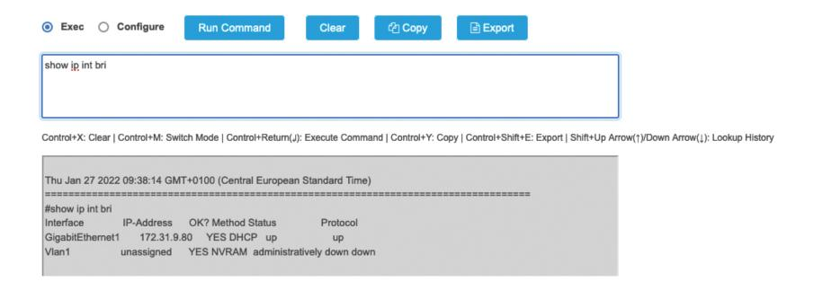
Figure 16-19 Command-line interface on the C9800 GUI
