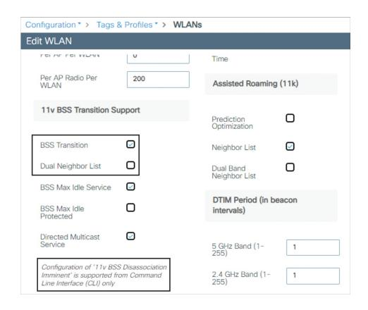
Figure 6-22 Configuring an 802.11v BSS transition on the C9800
