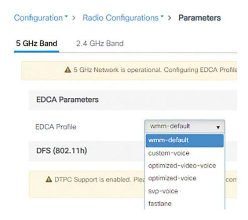
Figure 9-32 EDCA profile settings for a 5 GHz network
