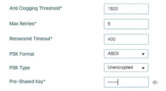
Figure 5-32 PSK configuration for SAE
