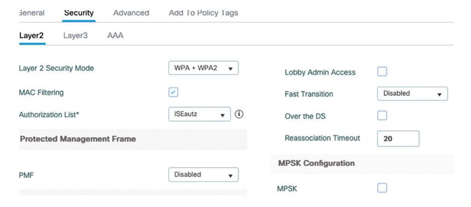
Figure 5-34 iPSK SSID security settings part 1
