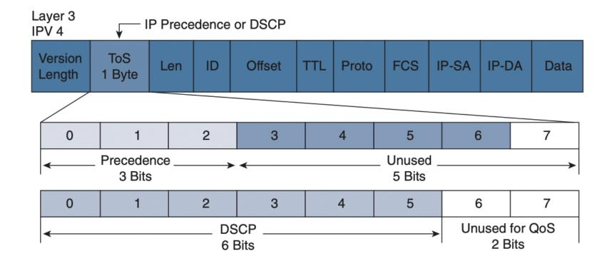
Figure 9-8 DSCP value in the IPv4 header
