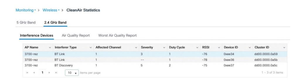
Figure 7-21 2.4 GHz CleanAir Interferer device report
