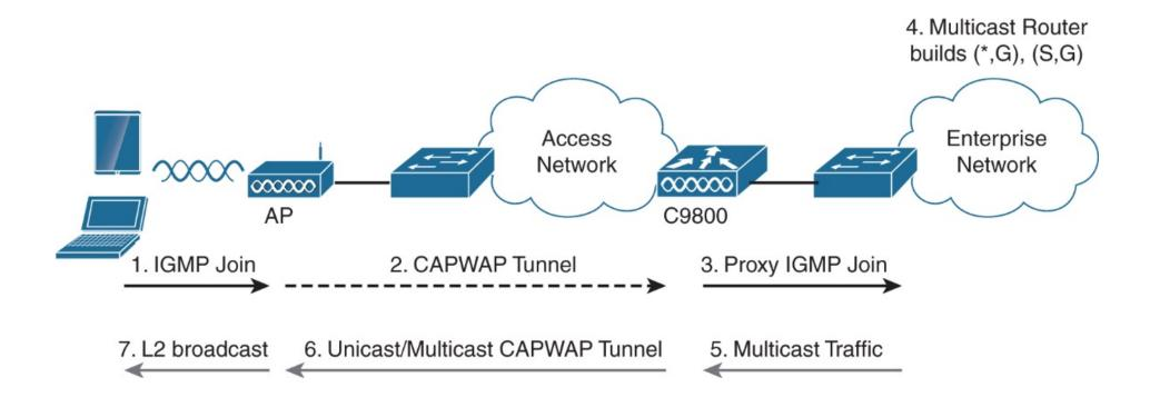
Figure 8-2 Multicast packet flow in wireless
