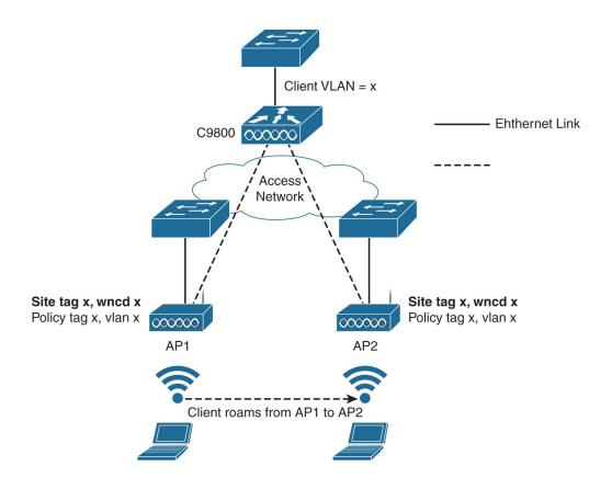
Figure 6-23 Intra-controller Intra-WNCd roaming on the C9800
