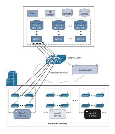
Figure 3-17 APs to WNCd distribution using custom site tag per roaming domain
