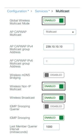
Figure 8-13 Configuring wireless broadcast and non-IP multicast forwarding
