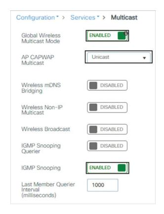
Figure 8-3 Enabling Multicast and MoU/MoM on the C9800
