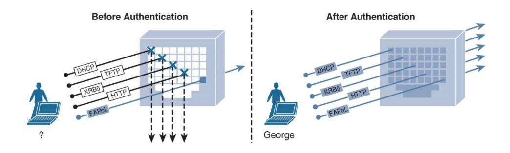
Figure 5-18 802.1X port-based authentication system
