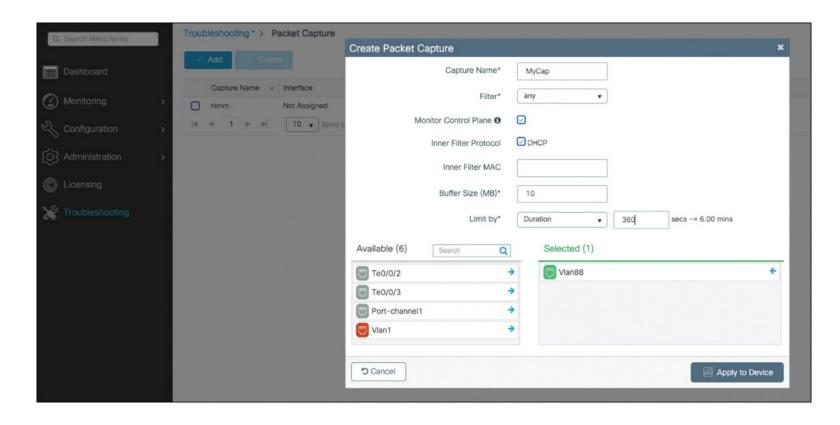
Figure 1-11 Defining a Packet Capture on C9800's GUI
