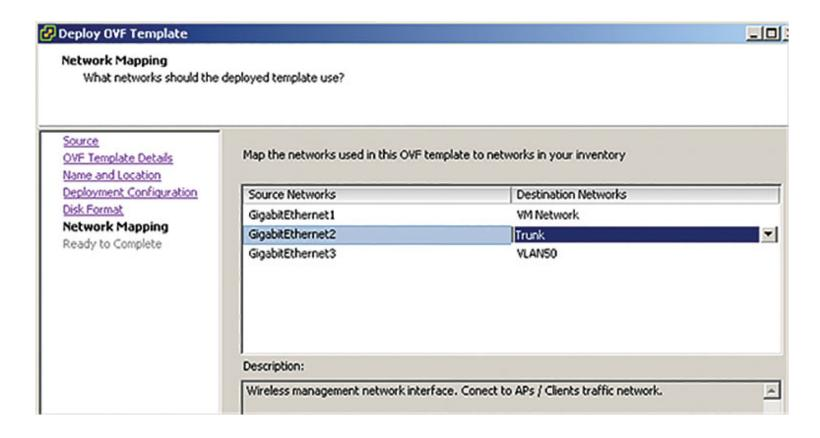
Figure 10-2 vNIC mapping for a C9800-CL over ESXi
