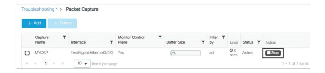
Figure 16-14 Monitoring progress and stopping EPC capture on the C9800 Troubleshooting dashboard
