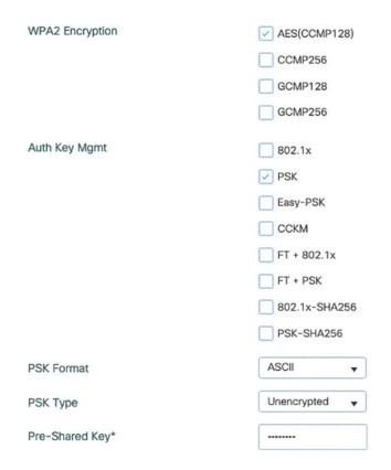
Figure 5-35 iPSK SSID security settings part 2
