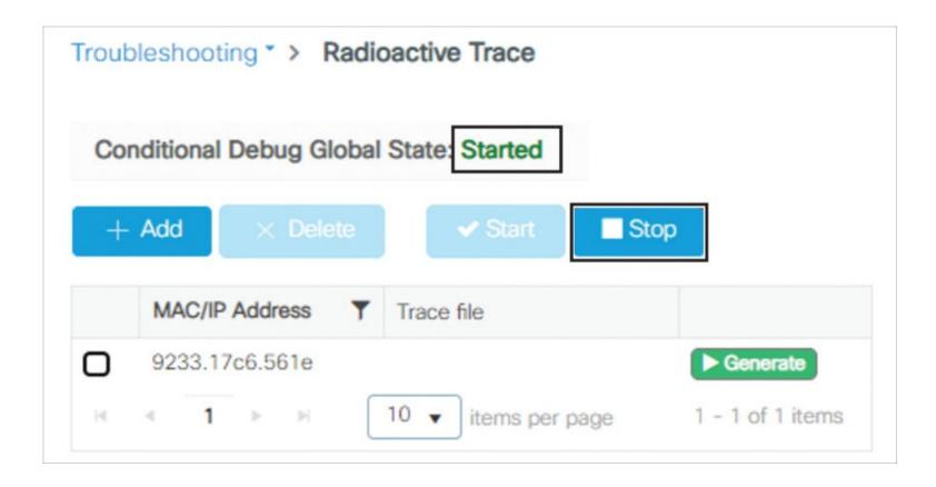
Figure 16-6 Starting a radioactive trace on the C9800 GUI
