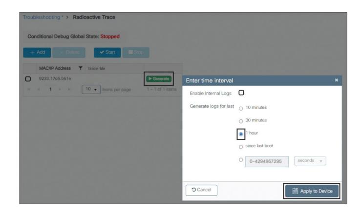
Figure 16-7 Collecting customer-use radioactive traces from the C9800 GUI
