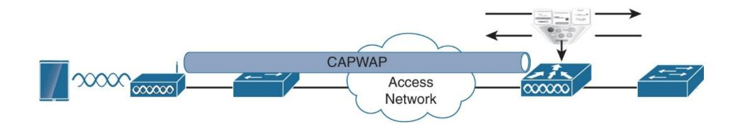
Figure 9-29 AVC in local mode and Flex central switching is applied at the WLC
