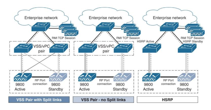
Figure 10-4 Supported topologies from an RP+RMI C9800 HA pair
