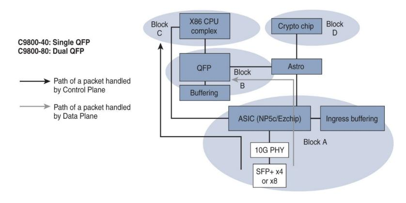
Figure 2-7 Block diagram of the life of a packet in the 9800 appliance's dataplane
