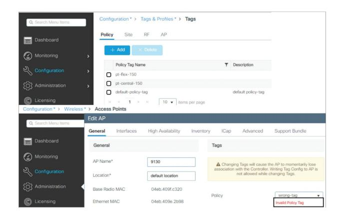
Figure 16-23 C9800 GUI preventing misconfiguration via configuration validation
