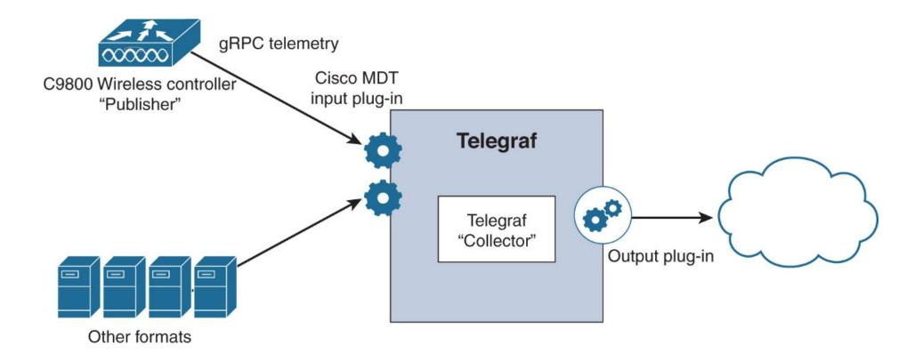
Figure 13-22 Telegraf serving as an aggregator for telemetry data
