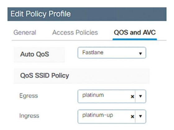
Figure 9-33 Recommended policy profile settings for an SSID with voice traffic
