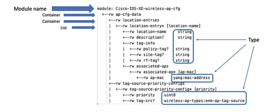
Figure 12-11 YANG module structure
