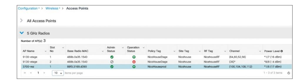
Figure 7-13 Manual channel configuration result
