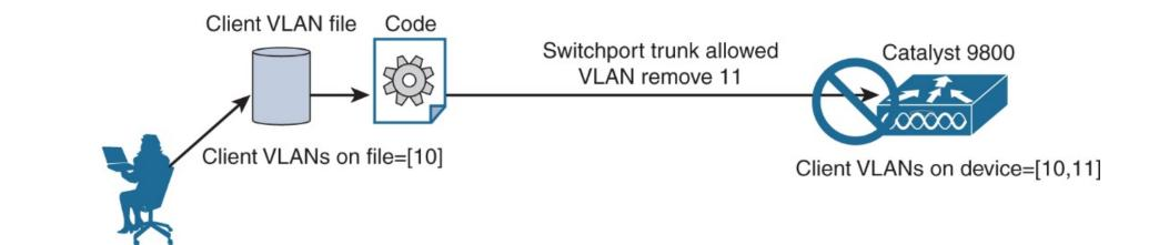
Figure 12-5 Errors when using imperative models
