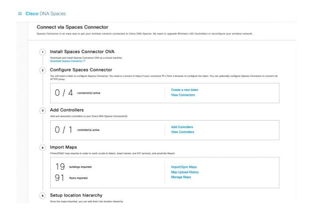
Figure 11-5 DNA Spaces Setup >Wireless page allowing you to generate tokens
