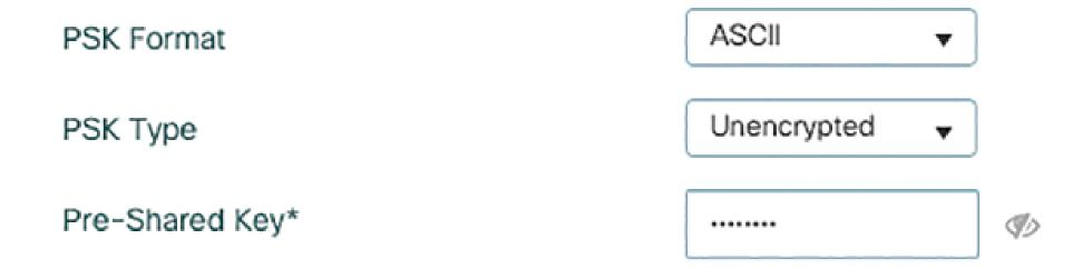
Figure 5-28 WPA2 PSK SSID key configuration
