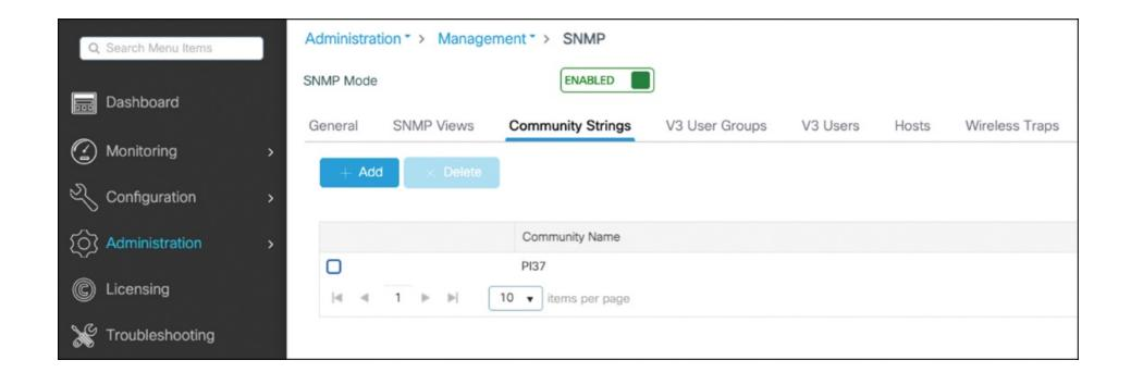
Figure 1-14 SNMP configuration of the C9800
