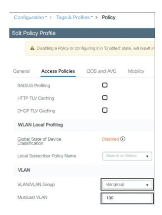
Figure 8-11 Configuring VLAN Select or multicast VLAN on the C9800 wireless policy profile
