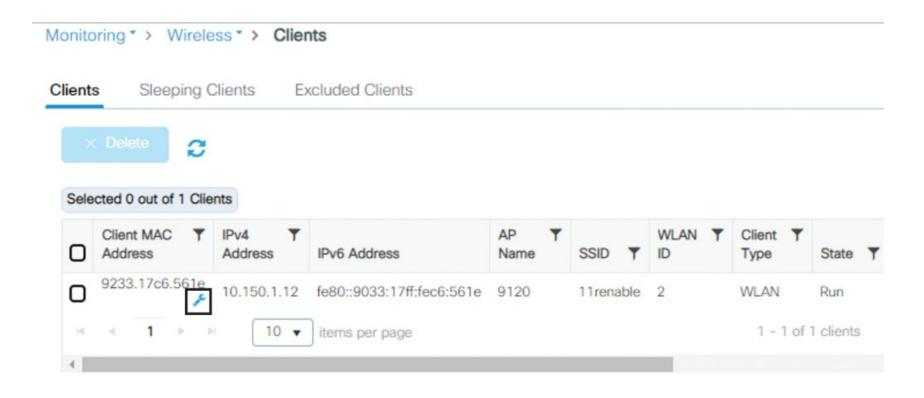
Figure 16-4 Selecting the client MAC address for conditional tracing from the client listed under Monitoring
