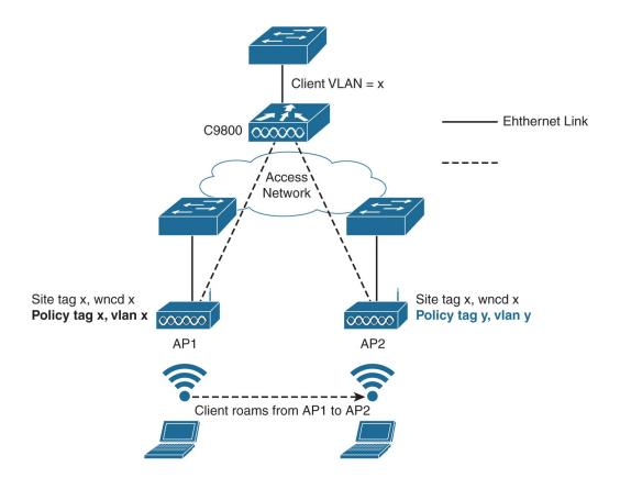
Figure 6-25 Intra-controller inter-policy profile roaming on the C9800
