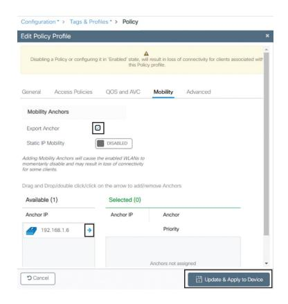
Figure 6-29 Configuring auto anchoring on the C9800
