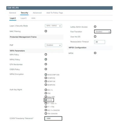
Figure 6-8 Configuring CCKM on the C9800
