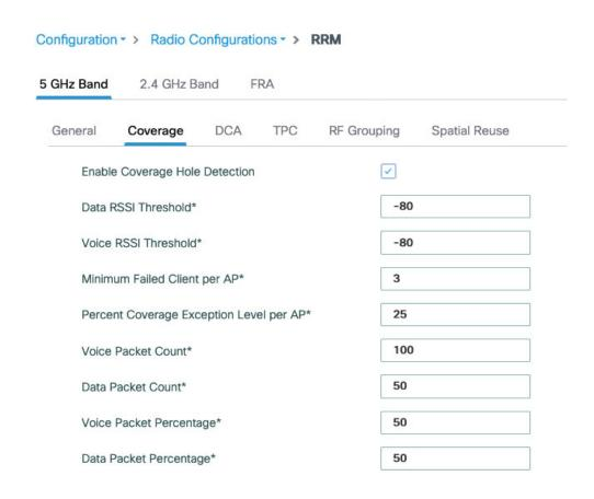
Figure 7-11 Coverage hole detection algorithm settings
