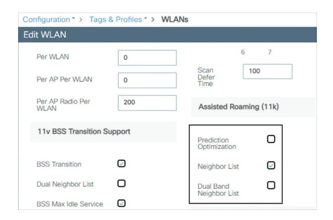
Figure 6-20 Configuring an 802.11k on the C9800 WLAN Profile
