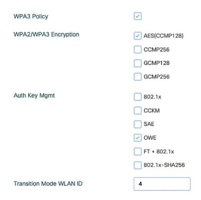
Figure 5-42 Enhanced Open SSID security settings part 2
