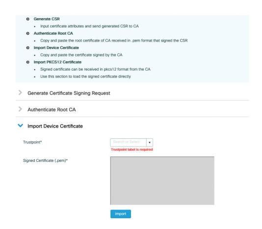
Figure 5-10 Adding the device signed certificate received from the CA
