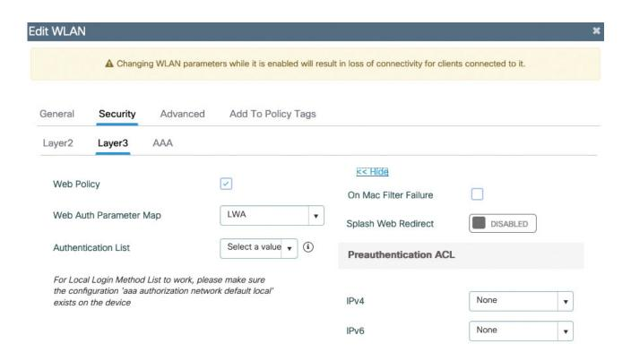
Figure 5-3 Layer3 WLAN security settings where the preauthentication ACL can be configured
