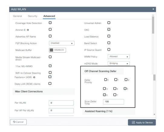
Figure 7-27 Off-Channel Scanning Defer setting
