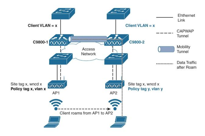
Figure 6-27 Layer 3 inter-controller roaming on the C9800
