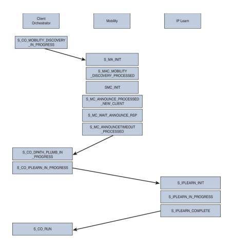
Figure 2-6 Client state machine on a WPA2 Enterprise SSID (continued)
