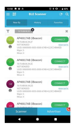
Figure 11-2 A BLE scanner application running on a smartphone
