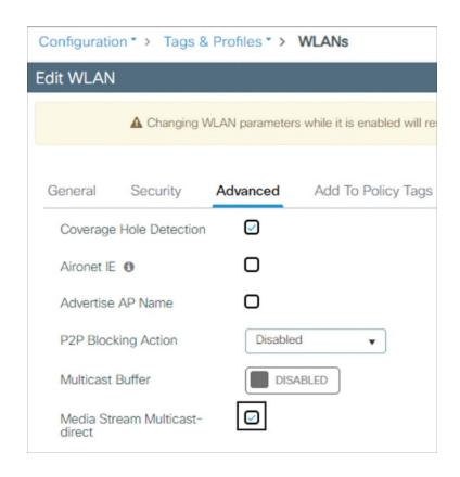
Figure 8-18 Enabling Media Stream on a client WLAN profile
