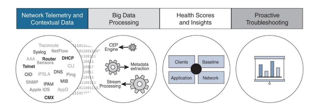
Figure 14-1 The principles of Cisco DNA Center telemetry and data processing flows
