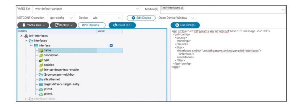
Figure 13-6 RPC to read configured interfaces using NETCONF
