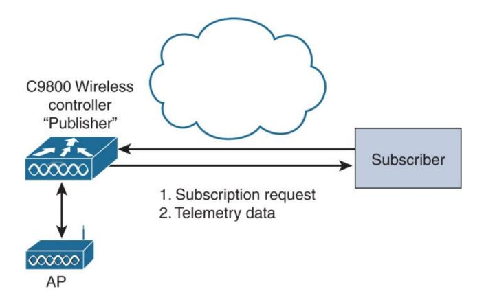
Figure 13-15 Flow for dial-in telemetry subscriptions
