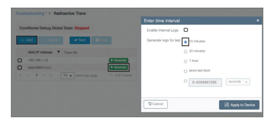
Figure 16-2 Collecting always-on traces for a client MAC from the C9800 GUI
