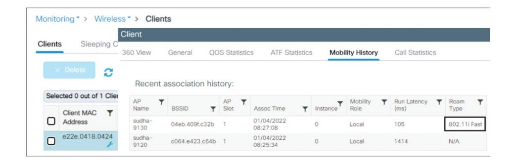
Figure 6-7 Monitoring the client roam type on the C9800
