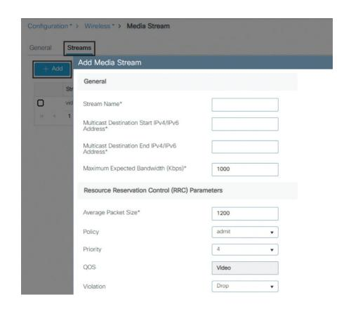
Figure 8-16 Configuring multicast stream details with their characteristics
