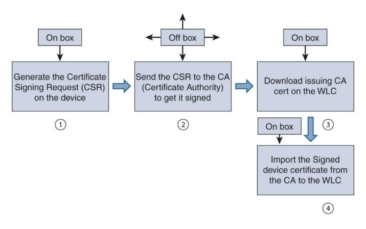
Figure 5-6 Adding a certificate by generating the question on the controller
