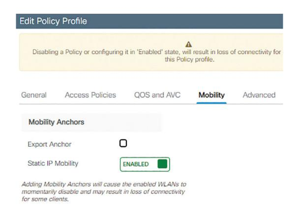
Figure 6-28 Configuring Static IP Mobility on the C9800
