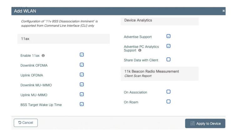
Figure 7-28 WLAN 11ax features configuration
