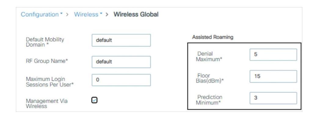
Figure 6-21 Configuring assisted roaming parameters on the C9800
