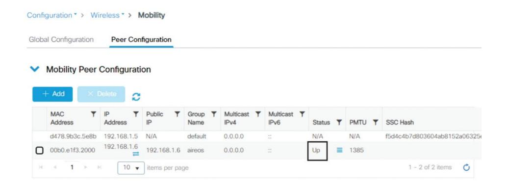
Figure 6-32 Monitoring mobility tunnel status on the C9800
