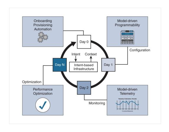
Figure 12-1 Programmability is used along all deployment phases
