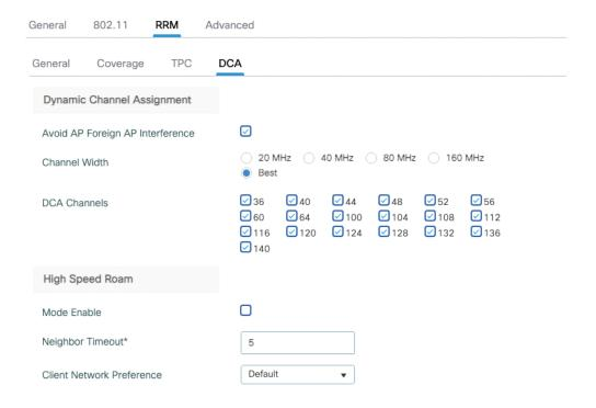
Figure 7-17 RF profile DCA configuration
