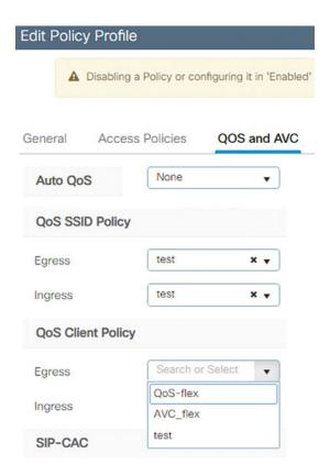
Figure 9-24 Assigning the policy at SSID or client level, or both
