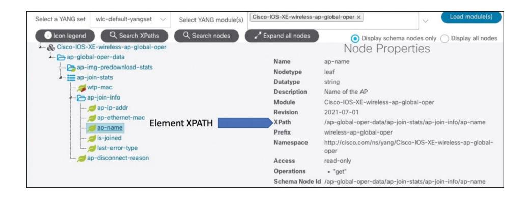
Figure 13-12 Element XPath as shown in YANG Suite
