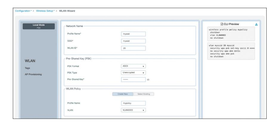
Figure 1-8 Setting up a PSK SSID with the WLAN Wizard
