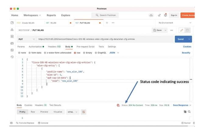
Figure 12-32 Replacing WLAN configuration using Postman
