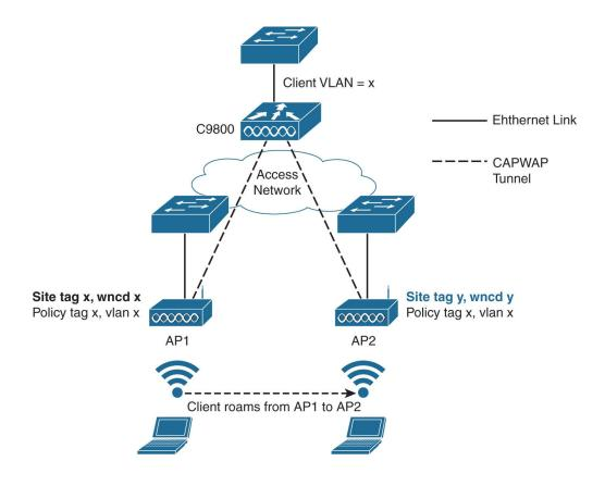
Figure 6-24 Intra-controller inter-WNCd roaming on the C9800
