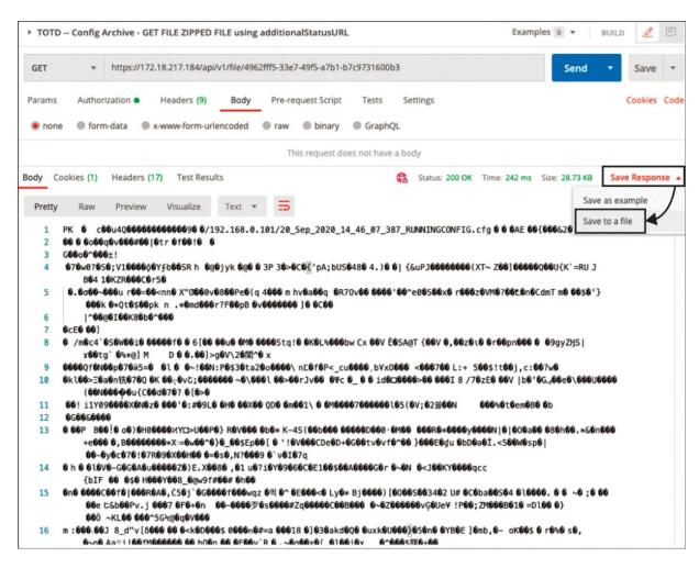
Figure 15-2 Saving the file containing the configurations through API calls
