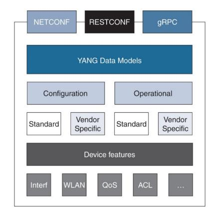
Figure 13-2 Configuration and operational YANG data models
