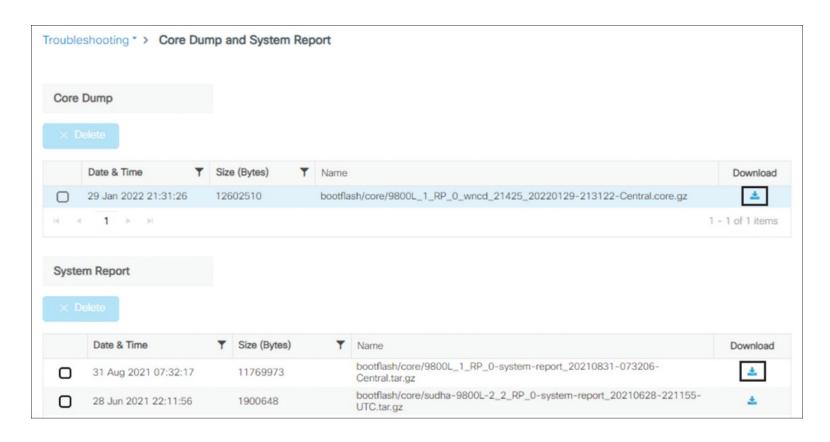
Figure 16-15 Core Dump and System Report web page that shows the WNCd core and two older system reports
