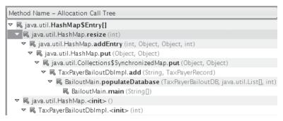
Figure 6-22 HashMap.Entry[] allocation stack traces
