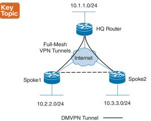
Figure 5-4 A Full-Mesh DMVPN Tunnel
