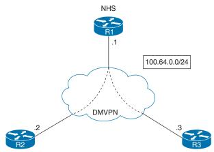
Figure 5-7 Basic DMVPN Hub-and-Spoke Example
