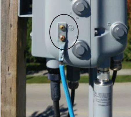
**Figure 4-8** *An Outdoor Access Point with Electrical Grounding (Photo Credit: Ian Procyk)*
