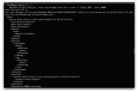
Figure 3-34 Using Python to Obtain the Entire Configuration of a Network Device
