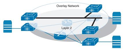
Figure 3-4 shows an example of an overlay network that provides Layer 2 capabilities.
