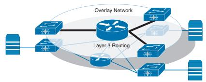
Figure 3-5 Overlay Network Providing Layer 3 Routing Capabilities
