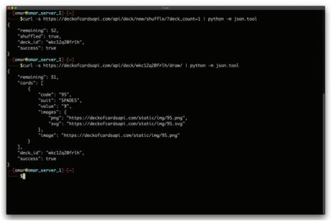
Figure 3-30 Using curl to Obtain Additional Information from the Deck of Cards API
