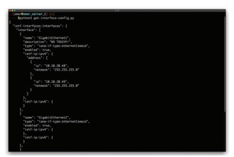
**Figure 3-35** Using Python to Obtain Information from a Network Device Using RESTCONF
