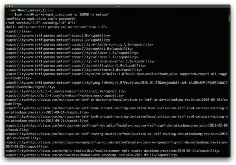
Figure 3-33 Using the NETCONF SSH Subsystem
