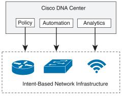
Figure 3-13 Cisco DNA High-Level Architecture
