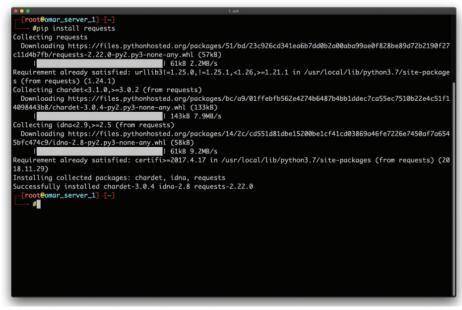
Figure 3-27 Installing the Python Requests Package Using pip
