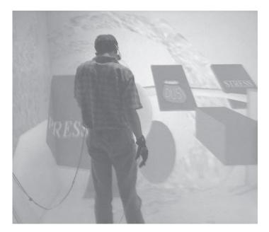
**Figure 9.17** Tool belt menu. Note that the tool belt appears larger than normal because the photograph was not taken from the user's perspective. (Photograph reprinted from Forsberg et al. [2000], © 2000 IEEE)
