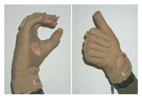
Figure 9.11 Examples of postures using a Data Glove. (Photograph courtesy of Joseph J. LaViola Jr.)
