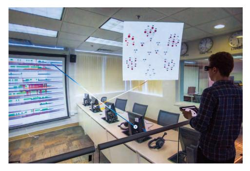
**Figure 9.6** Tablet control of interactive visualizations layered on top of surround-view imagery in the UCSB Allosphere. Photograph shows left-eye view of stereo content viewed and controlled by the user. (Image courtesy of Donghao Ren and Tobias Höllerer)
