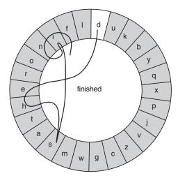
Figure 9.16 Layout of the Cirrin soft keyboard for pen-based input (Mankoff and Abowd 1998, © 1998 ACM; reprinted by permission
