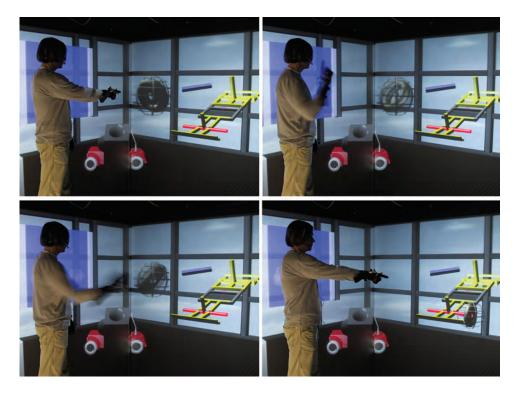
Figure 9.21 A car wheel is selected, rotated, and moved to its correct position using voice and gestures. (Photographs courtesy of Marc Eric Latoschik, AI & VR Lab, University of Bielefeld; Latoschik 2001)
