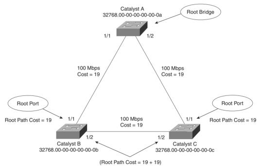
The Root Bridge, Catalyst A, already has been elected. Therefore, every other switch in the network must choose one port that has the best path to the Root Bridge. Catalyst B selects its port 1/1, with a Root Path Cost of 0 plus 19. Port 1/2 is not chosen because its Root Path Cost is 0 (BPDU from Catalyst A) plus 19 (Path Cost of A–C link), plus 19 (Path Cost of C–B link), or a total of 38. Catalyst C makes a similar choice of port 1/1.
