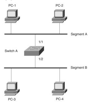
Figure 9-1 Transparent Bridging with a Switch
