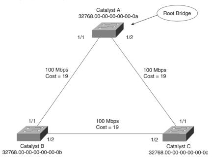
In this network, each switch has the default Bridge Priority of 32,768. The switches are interconnected with Fast Ethernet links. All three switches try to elect themselves as the Root, but all of them have equal Bridge Priority values. The election outcome produces the Root Bridge, determined by the lowest MAC address—that of Catalyst A.
