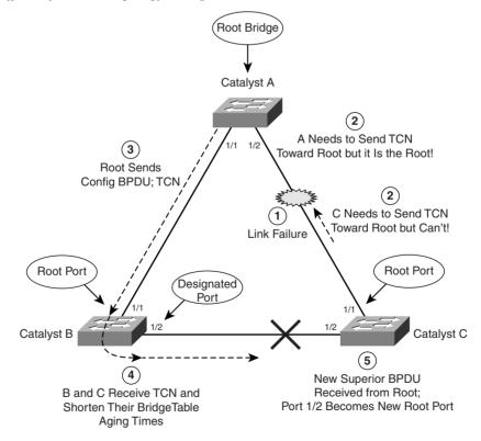
This network has just suffered a link failure between Catalyst A and Catalyst C. The sequence of events unfolds as follows:
