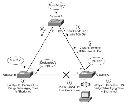
Obviously, user ports are expected to go up and down as the users reboot their machines, turn them on and off as they go to and from work, and so on. Regardless, TCN messages are sent by the switch, just as if a trunk link between switches had changed state.
