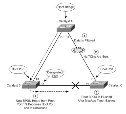
STP can detect and recover from indirect failures, thanks to timer mechanisms. The sequence of events unfolds as follows:
