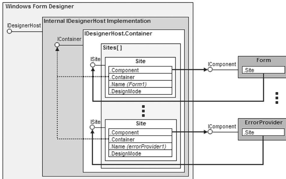
FIGURE 9.5: Design-Time Architecture
