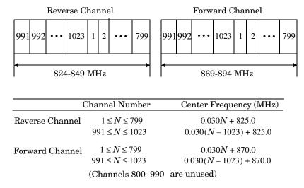
**Figure 1.2** Frequency spectrum allocation for the U.S. cellular radio service. Identically labeled channels in the two bands form a forward and reverse channel pair used for duplex communication between the base station and mobile. Note that the forward and reverse channels in each pair are separated by 45 MHz.
