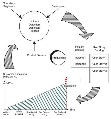
**Figure 2.4** *Process for reducing customer escalations*
