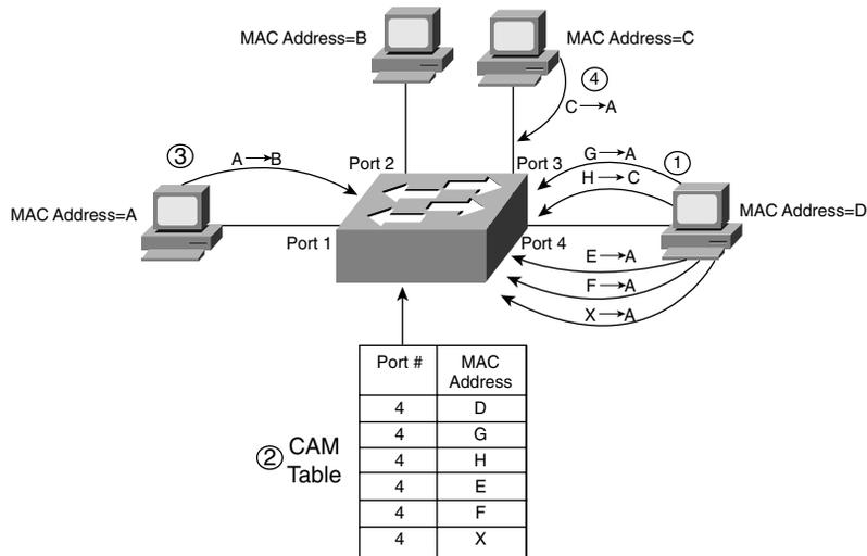
Figure 5-1 shows a series of steps that take place to orchestrate a MAC address flooding attack. Given below is the list of steps that takes place as shown in the Figure 5-1:
