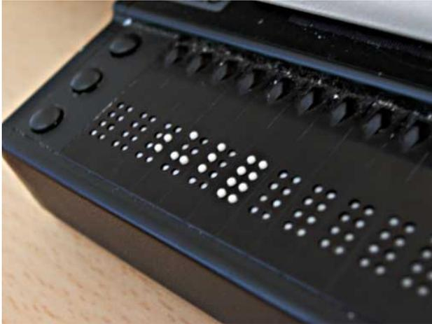
**FIGURE 5-1** The refreshable Braille display
