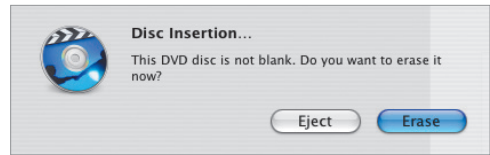
Figure 5.14 If you insert a rewriteable disc that contains data, iDVD can erase it during the burn stage.
