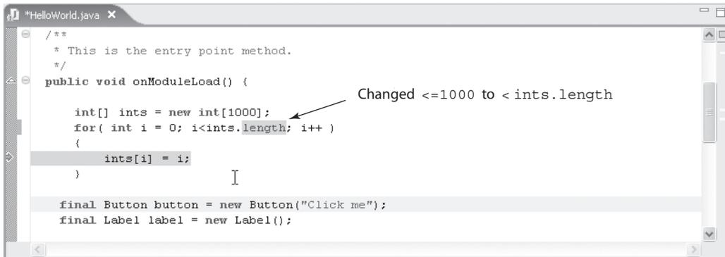
**Figure 4-30.** Fixing the code while debugging
