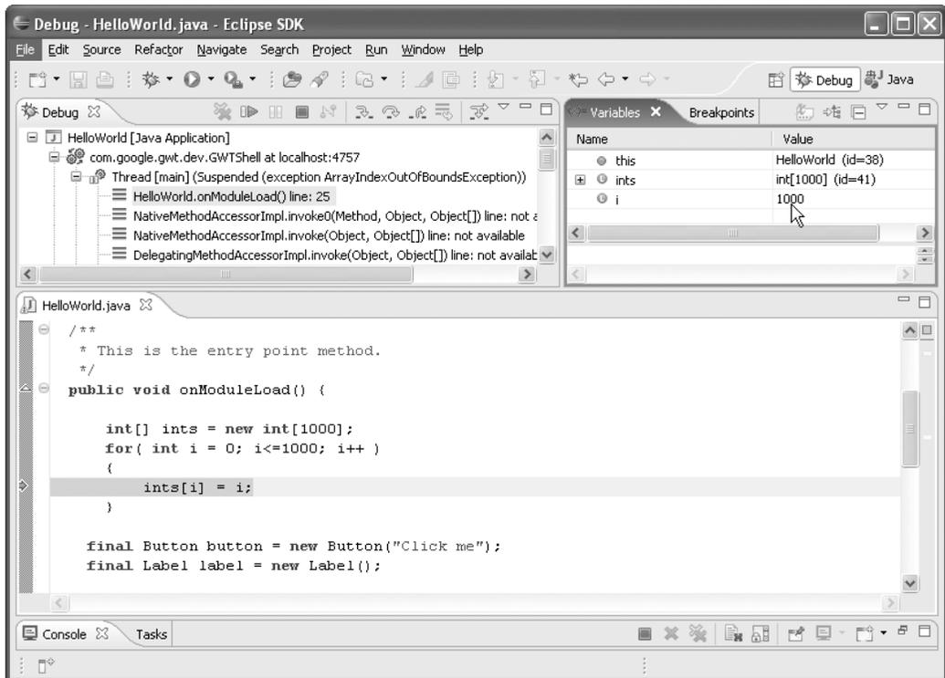
**Figure 4–29.** Breaking into the debugger on an exception
