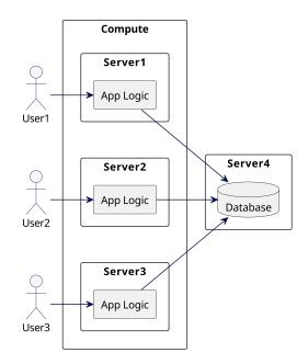
Figure 1.4 Scaling compute with multiple servers
