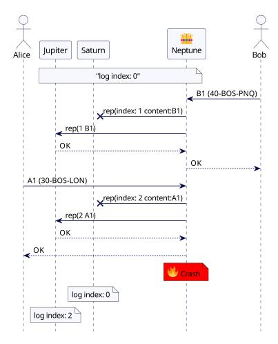
**Figure 2.12** Leader failure—incomplete replication—using log
