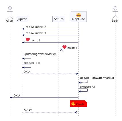
Figure 2.24 The High-Water Mark is propagated using HeartBeat.
