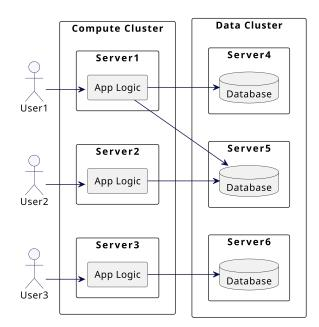
Figure 1.5 Scaling data by distributing on multiple servers
