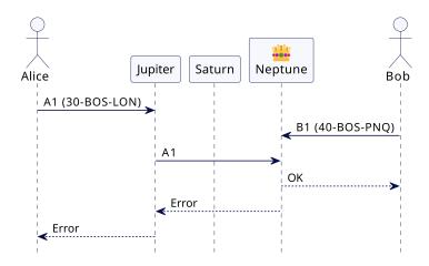
Figure 2.8 Leader rejecting requests for insufficient widgets
