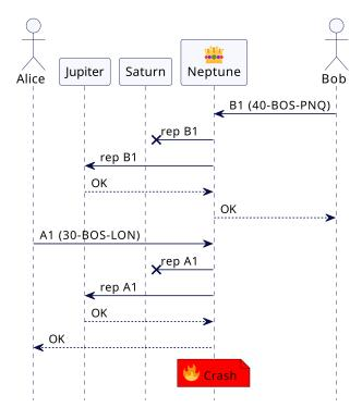
Figure 2.11 Leader failure—incomplete replication
