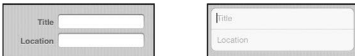
Figure 3.10 Text fields (left) look dated, feel cramped, and are hard to balance. A table cell with text input enabled looks nicer, and using placeholder text instead of a value cell style leaves more room for typing.
