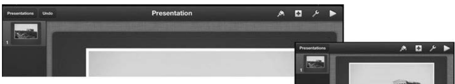
Figure 3.7 Keynote has similar toolbar configurations on iPad and iPhone. Bordered and unbordered buttons are kept separate for the sake of tidiness.
