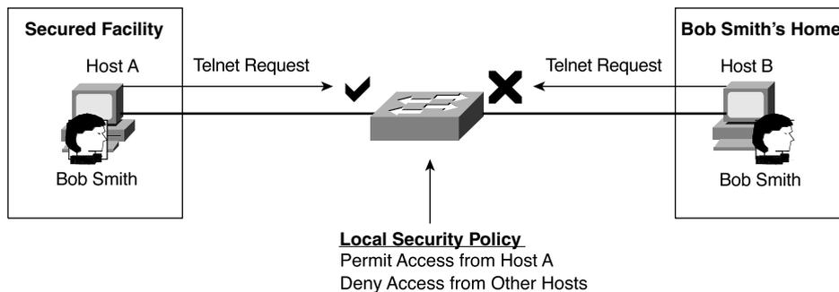
Through the use of permit lists on CatOS and access classes on IOS, management sessions can be controlled on a source IP address basis for the following protocols:
