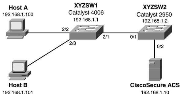
A Catalyst 4006 (XYZSW1) provides access for Hosts A and B. Host A is a dedicated network administration workstation that is used to manage the network. Host B is a user's PC, and should not be allowed management access to any network devices. A Catalyst 2950 (XYZSW2) provides connectivity to the company servers, including a recently installed CiscoSecure asynchronous communications server (ACS). Both switches are interconnected by a single Fast Ethernet trunk.
