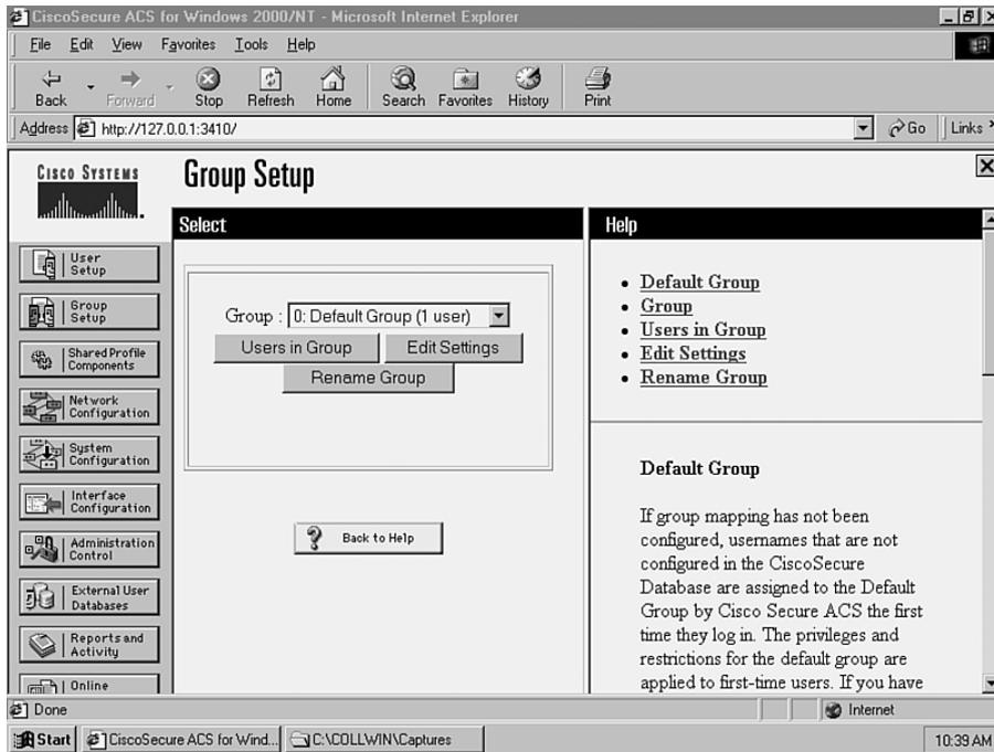
**Step 2** On the Group Setup page, scroll down to the *TACACS+ Settings* section and enable the Shell (exec) setting and configure Privilege level to be 15 (enable mode), as shown in Figure 8-10. This authorizes the user for enable mode (privilege level 15) access via TACACS+.
