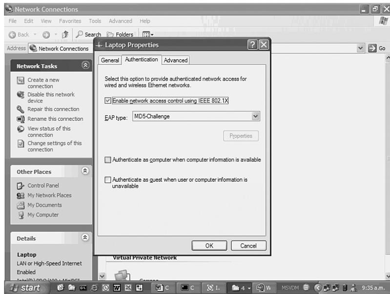
**Step 3** Connect the LAN interface to XYZSW1 port 2/3. You should receive a notification, asking you to authenticate LAN access, as shown in Figure 8-19. Enter *administrator* as the username and *password* as the password, leaving the domain field blank.
