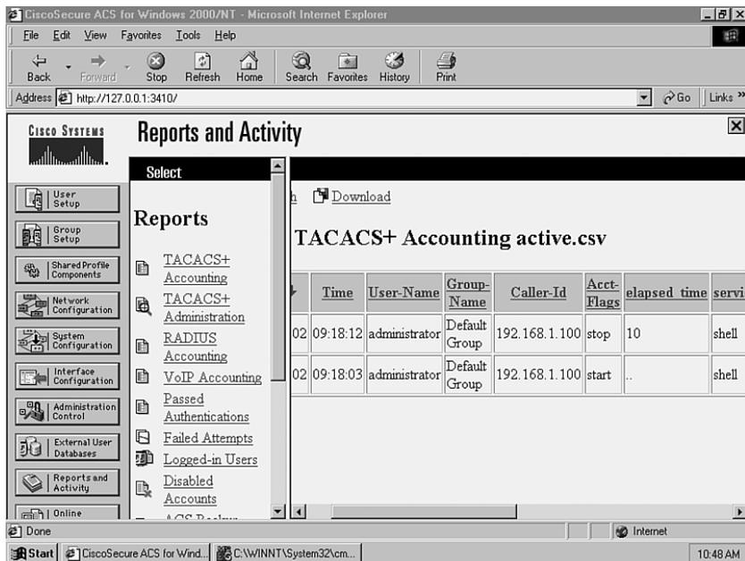
Figure 8-14 shows a start and stop record around 09:18 a.m. The *Service* column indicates this is a *shell* (exec) event, and the *elapsed time* column for the *stop* record indicates the session lasted for 10 seconds. The *User-Name* column indicates that the user *administrator* established the exec connection, and the *Caller-Id* column indicates that the exec session was initiated from 192.168.1.100 (Host A).
