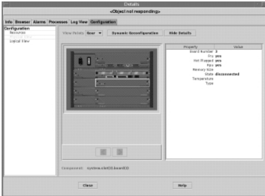
Figure 4-5 Using the SyMON Physical View to identify a failed hardware component.
