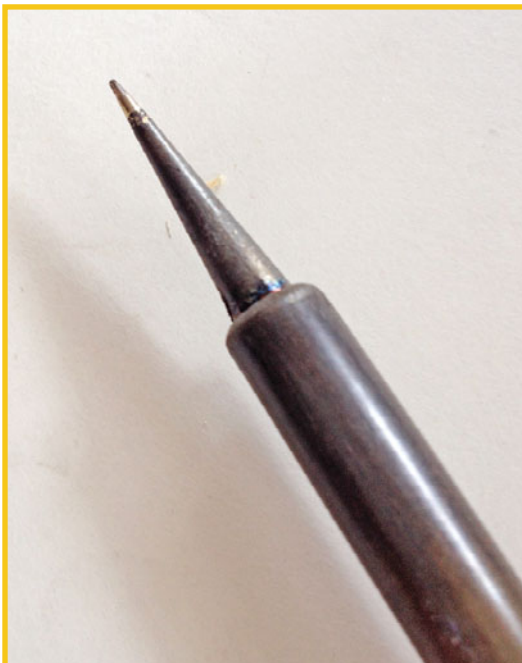
FIGURE 4.12 Coat the tip of your iron with solder.
