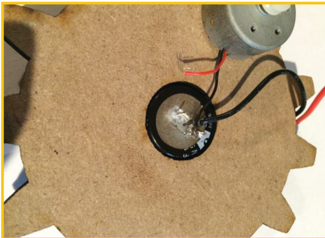
FIGURE 4.28 Connect the negative leads of the three components.
