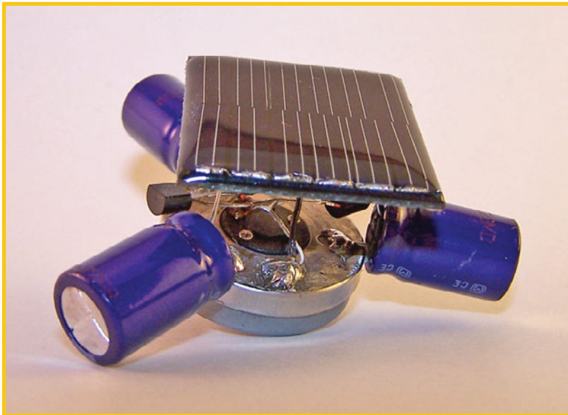
FIGURE 4.3 This solar-powered robot spins when light strikes it.
